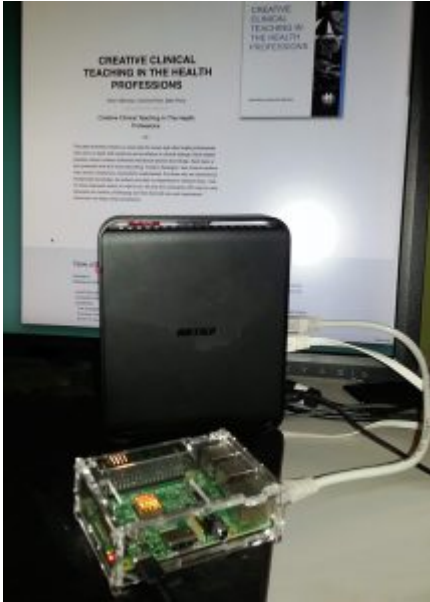
Raspberry Pi 3 Model B hardwired to WiFi Router with desktop display of resulting Pressbooks server book site.
